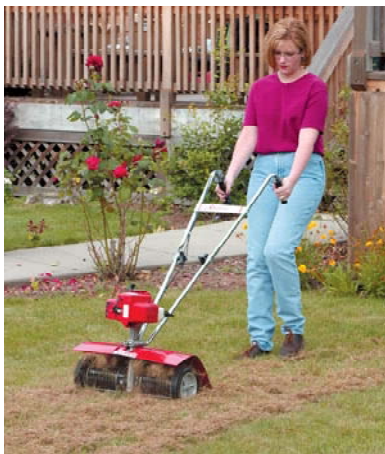
For the smaller property or niche area, the right turf care tool may be a tiller with applicable attachment. Handheld tiller above, shown with dethatcher attachment.
