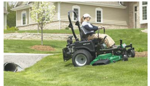
23-inch drive wheels and 49-inch stance provide exceptional traction, handling and stability.
