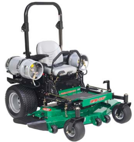
New Predator-Pro LP (above) shown with side discharge deck and optional ROPS.
