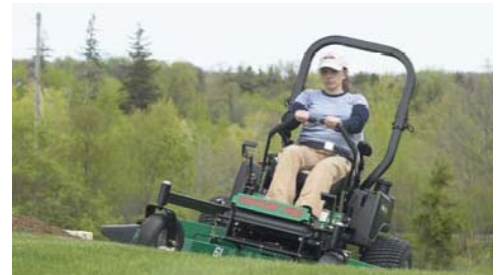
23-inch drive wheels and 49-inch stance provide exceptional traction, handling and stability.
