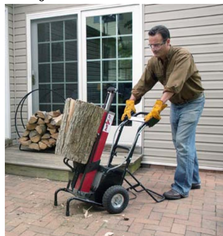
Some vertical units utilize a dolly chassis design making them as easy to wheel around as a suit case.
